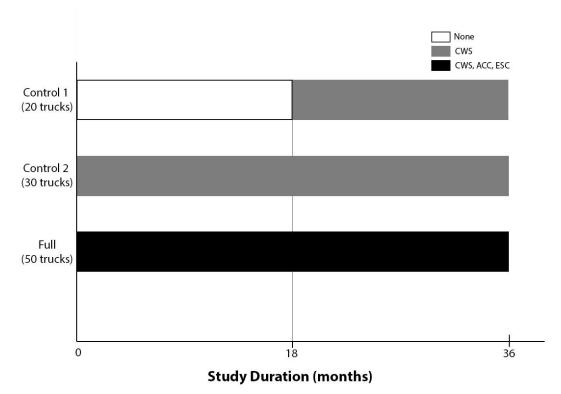
Figure 3. Design of the DOT and Volvo study showing three groups testing different forward CAS technologies (key at top right of graphic) over various time frames.
