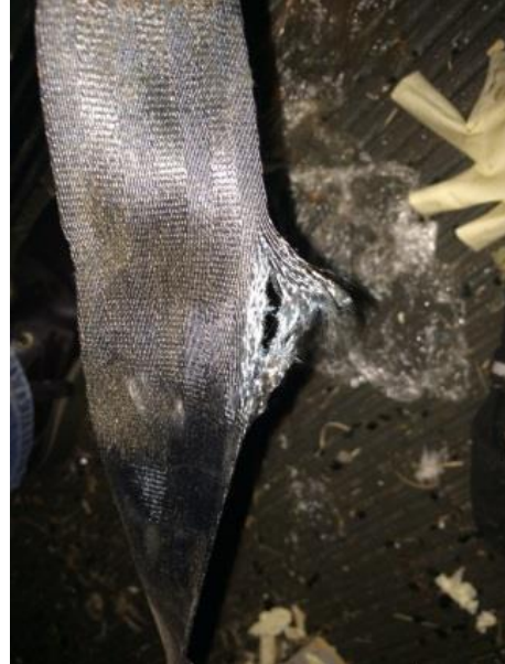
Figure 2. Seat belt with webbing torn in a location similar to where other belts were trapped.
