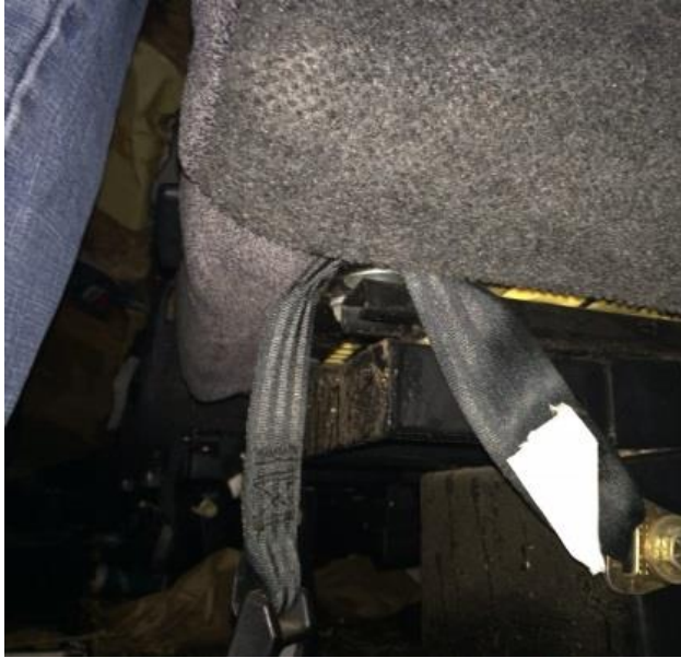
Figure 1. Seat belt webbing pinched by the side-sliding seat track.
