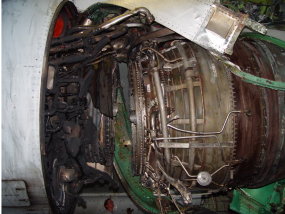
Figure 2. View of the left side of the No. 1 engine showing the engine split in two.
