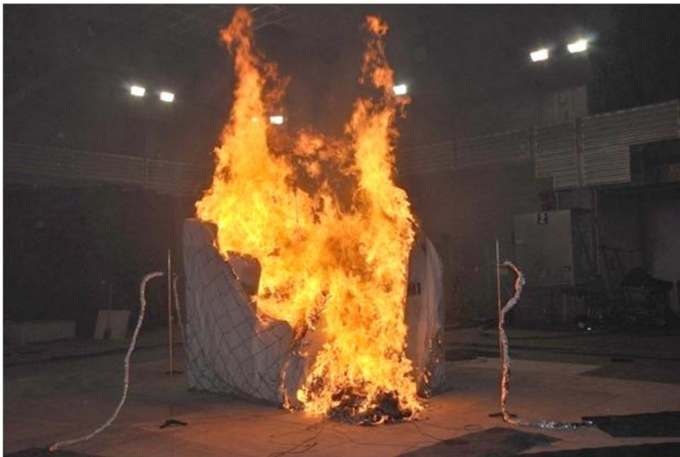
Figure 1. Photo taken during the NTSB cargo container fire study depicting a polypropylene cargo container burning at a rate of 8.45 megawatts (MW), 132 seconds after becoming detectable to an aircraft-based smoke detection system.
