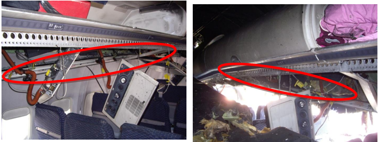
Figure 4. Photographs showing failed aircraft rail on the left and right side of the aft section of Continental Airlines flight 1404.
