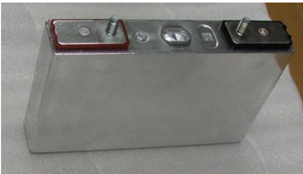
Figure 2. Individual 90 Wh cell removed from the battery module.
