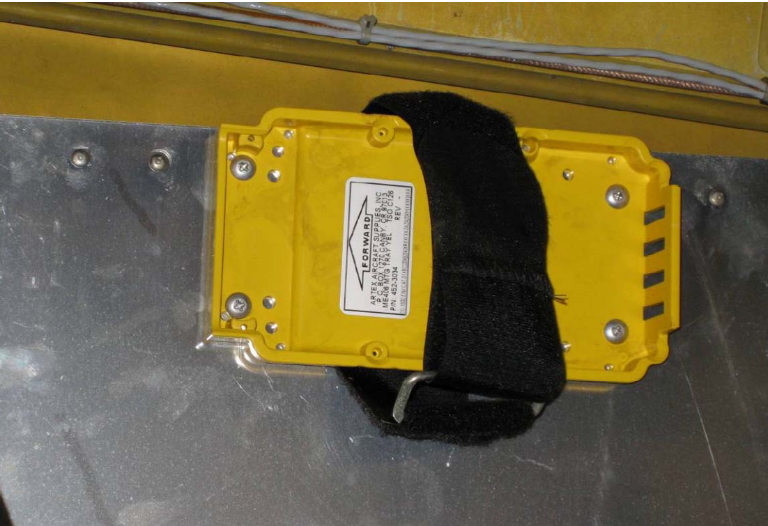
Figure 1. ELT tray with webbed strap mounted on sidewall of accident airplane.
