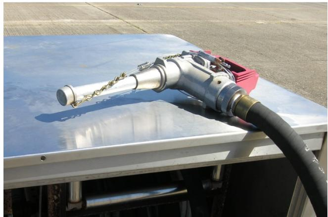
**Figure 1.** Photograph of an avgas nozzle.
