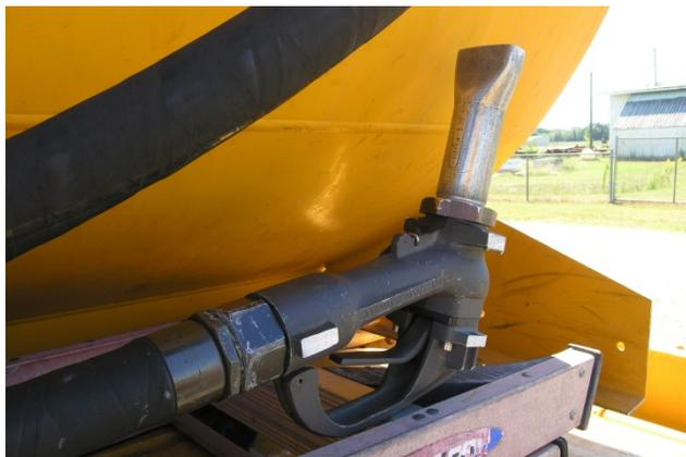
**Figure 2.** Photograph of Jet A fuel nozzle.
