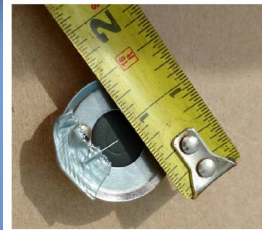
Obstruction to the Valve Seat
