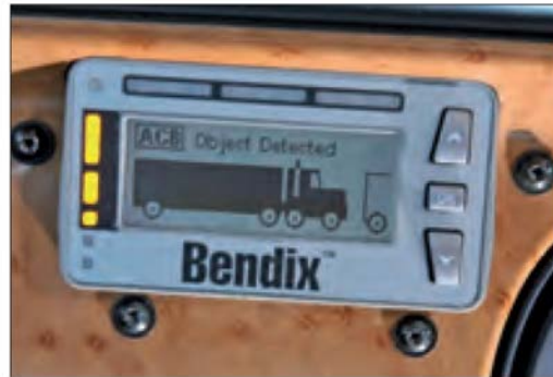
Example of Stationary Object Alert Display
