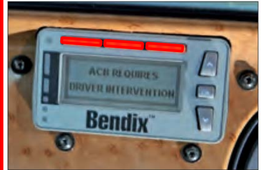
Example of Impact Alert Warning Display
