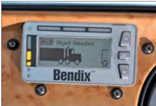
Example of Following Distance Alert Display
