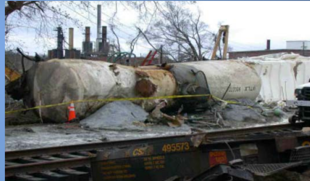
Ruptured Chlorine Tank Car, Graniteville, South Carolina
