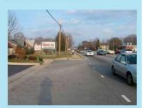
The sidewalk in this photograph terminates in a right turn lame. Pedestrians must contend not only with right turning traffic, but traffic crossing their paths at the two access points located off of the lame. Motorists exiting these driveways are focused on finding a gap in traffic and avoiding conflicts with right turning vehicles and may not see pedestrians walking along the side of the road. The RSA team may suggest providing a continuous, level sidewalk through this area.
