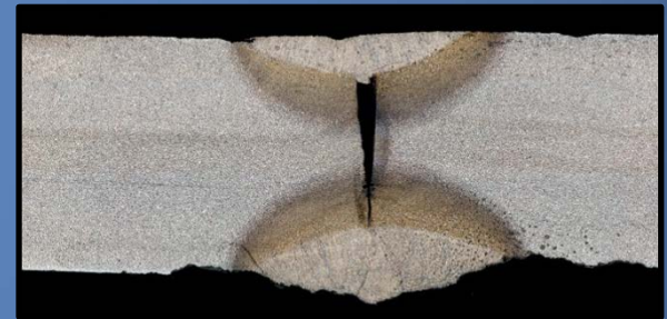
Manufacturing (bad weld)
