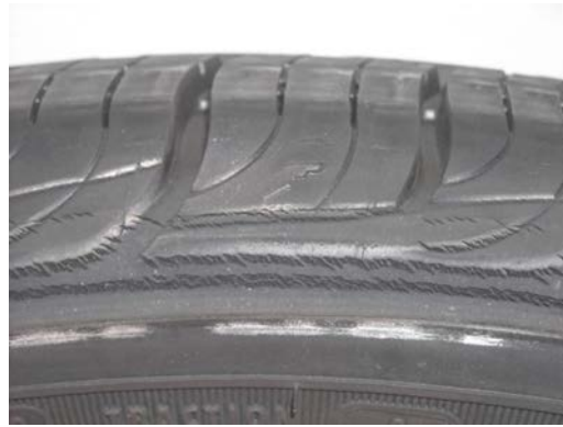
Cracking in shoulder
