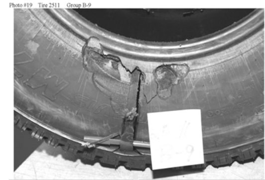
Sidewall split and rupture
