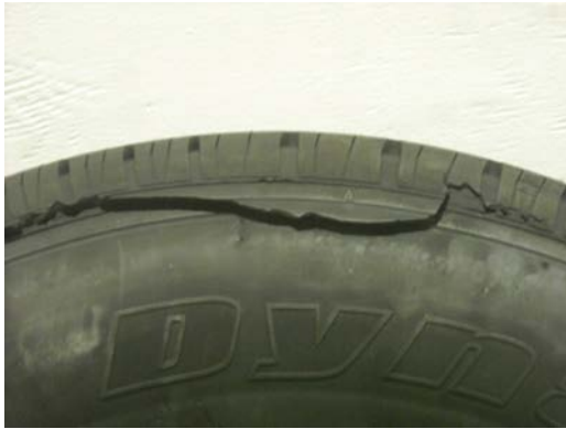
Tread separation at shoulder
