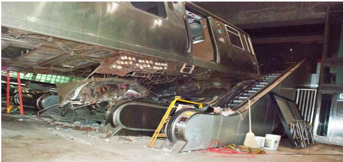
Figure 1. Damaged train No. 141 resting on the escalator.
