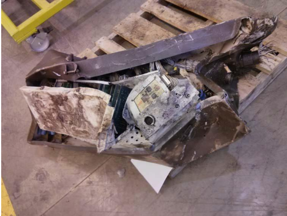
Figure 8. The card rack, which recorded the event data, was within the undercarriage and was damaged in the crash.
