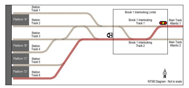
**Figure 2.** Diagram of tracks at Atlantic Terminal. (Brook 2 is to the right of Brook 1 and is not shown in the figure.)
