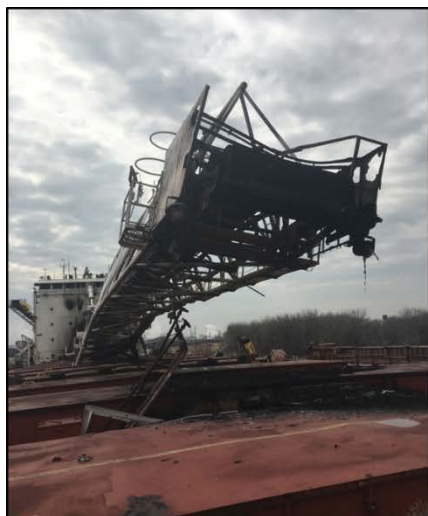
Fire damage to the vessel: (left) cargo conveyor boom, (center) stern of the deckhouse, and (right) the bridge.
