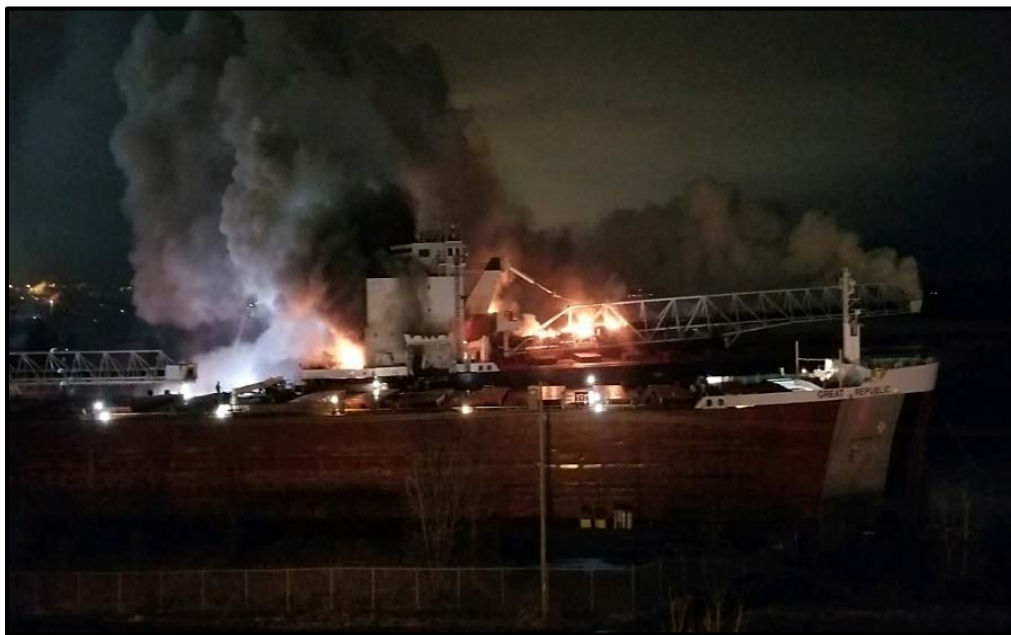
Vessel fire at 2209. Billowing smoke pours from the vessel as fire in the aft part of the deckhouse spreads up the conveyor belt on the boom. (Source: Great Lakes Trader Chief Engineer)
