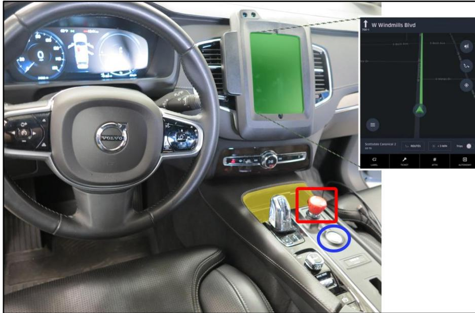
**Figure 6.** SUV interior showing locations of slot that could mount a cell phone (yellow region in center console), ADS engagement/disengagement knob (red), ADS engagement button (blue), and HMI (with inset illustrating image on tablet).
