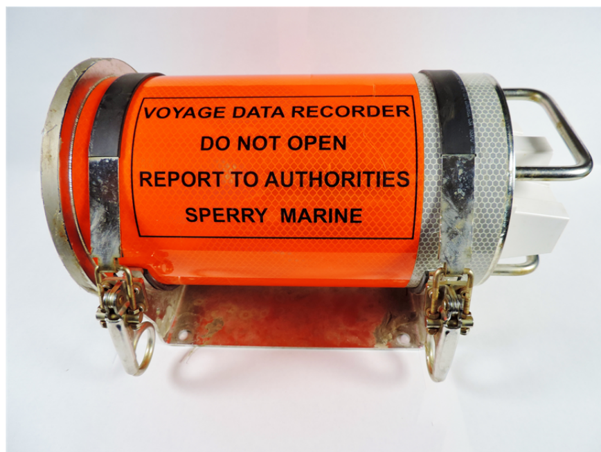
Exemplar fixed capsule for the S-VDR installed on the El Faro.
