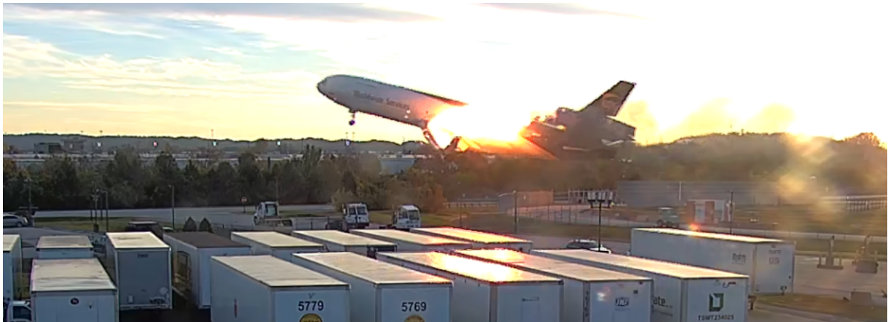
Figure 2. The fire in the area of the left pylon attachment to the wing continued as the airplane cleared the blast fence.
