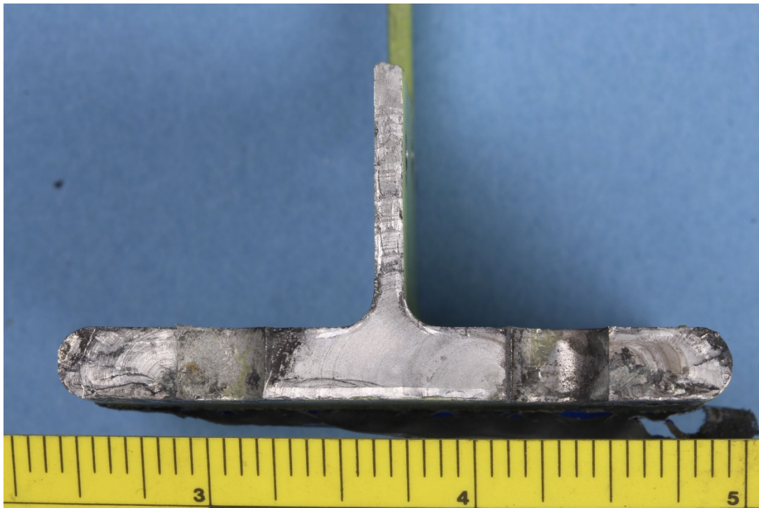
Figure 1 – Left wing main spar lower cap fracture surface.
