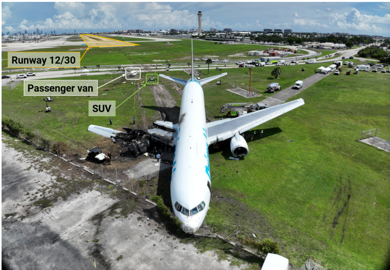
Figure 6. An aerial view of N1997A showing the relative location of the two impacted ground vehicles and ground scars leading up to the airplane's resting location.
