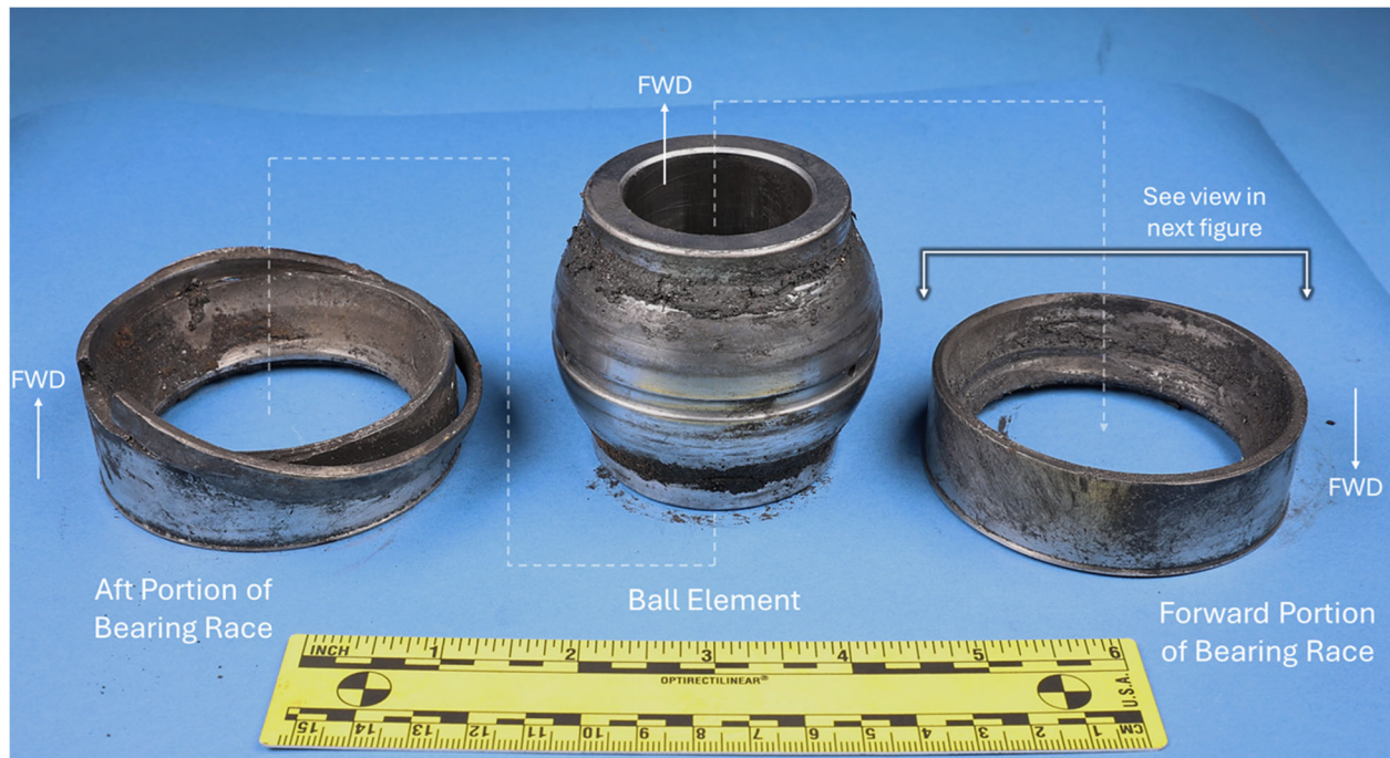
Figure 2. The accident spherical bearing assembly from the left pylon aft mount bulkhead showing the bearing race fractured into forward and aft portions.
