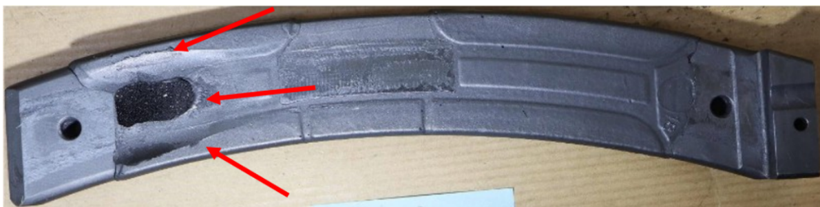
Figure 8. No. 10 spacer damage (Source Safran Aircraft Engines).
