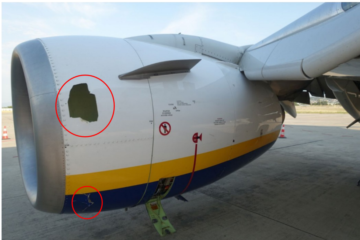
Figure 5: No. 2 (right) engine inlet cowl outer barrel punctures.
