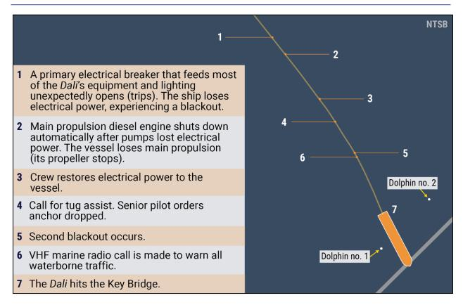
**Figure 7.** The *Dali*'s route on March 26, between the first blackout, and the *Dali* striking pier no. 17 of the Key Bridge. The location and approximate size of two of the bridge's "dolphins," sheet pile and concrete structures protecting the bridge's piers, are labeled in the lower right.
