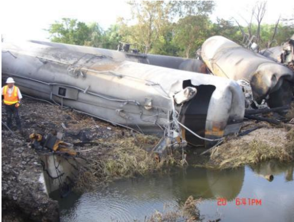
Figure 10. Breach in tank car NATX 303504. (Federal Railroad Administration photo)
