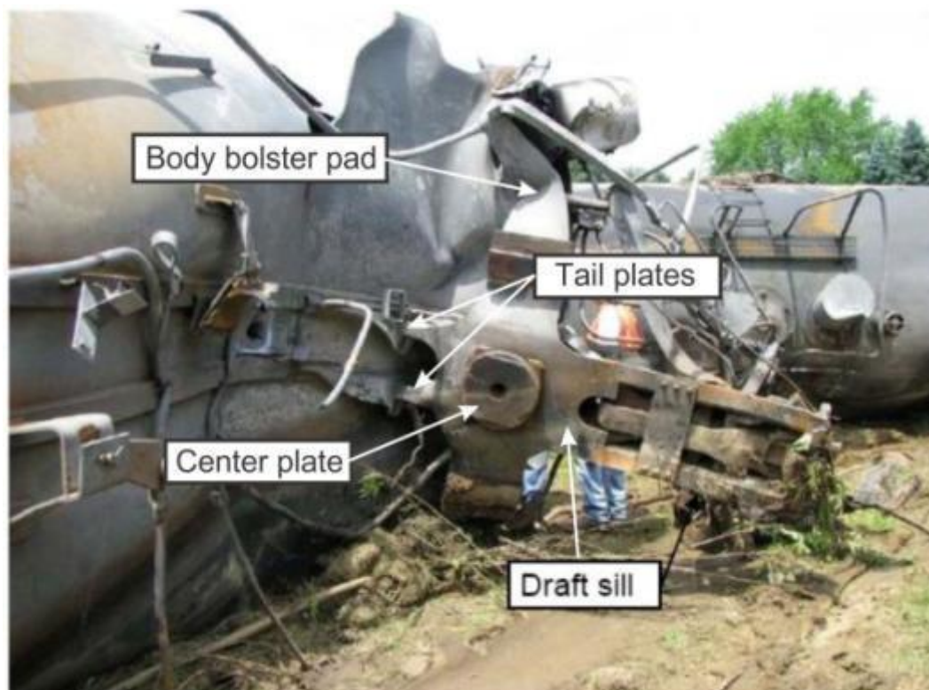
Figure 21. Underside of B end of tank car NATX 303504 as viewed from A end.
