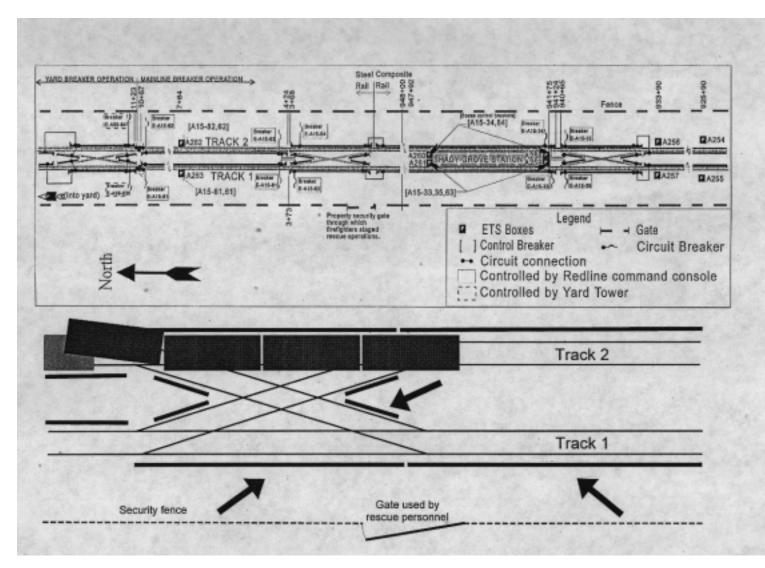
Figure 12 – Schematic representations (not to scale) of Metrorail third rail power control in the accident area. Arrows in the lower illustration indicate third rail sections that remained energized for 43 minutes after the accident.
