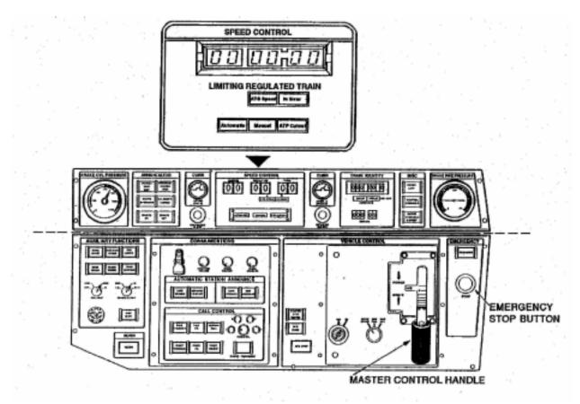
Figure 3 – The operator's console on both Breda and Rohr Metrorail cars is a two-part console divided into a sloping indictor panel and a flat control panel section. The speed control blowup illustrates the Breda configuration.
