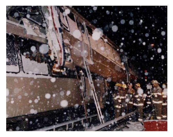
Figure 5 – Final position of accident trains. Gap train (left) has telescoped 21 feet into the shell of train T-111
