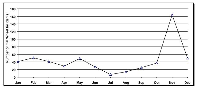
Figure 10 – Flat wheel incidents occurring in 1995 and resulting in multiple wheel flats. *Source:* Metrorail maintenance and reliability system (MARS) significant incident report provided at Safety Board request.
