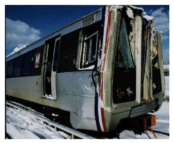
Figure 7 -- Head end (struck end) of gap train
