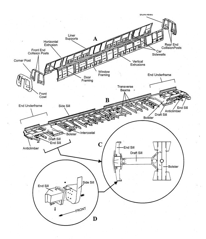
Figure 8 – (A) Typical WMATA Metrorail carbody structure; (B) Underframe of Breda Metrorail car; (C) End underframe assembly; (D) Attachment of side sill to end sill of underframe
