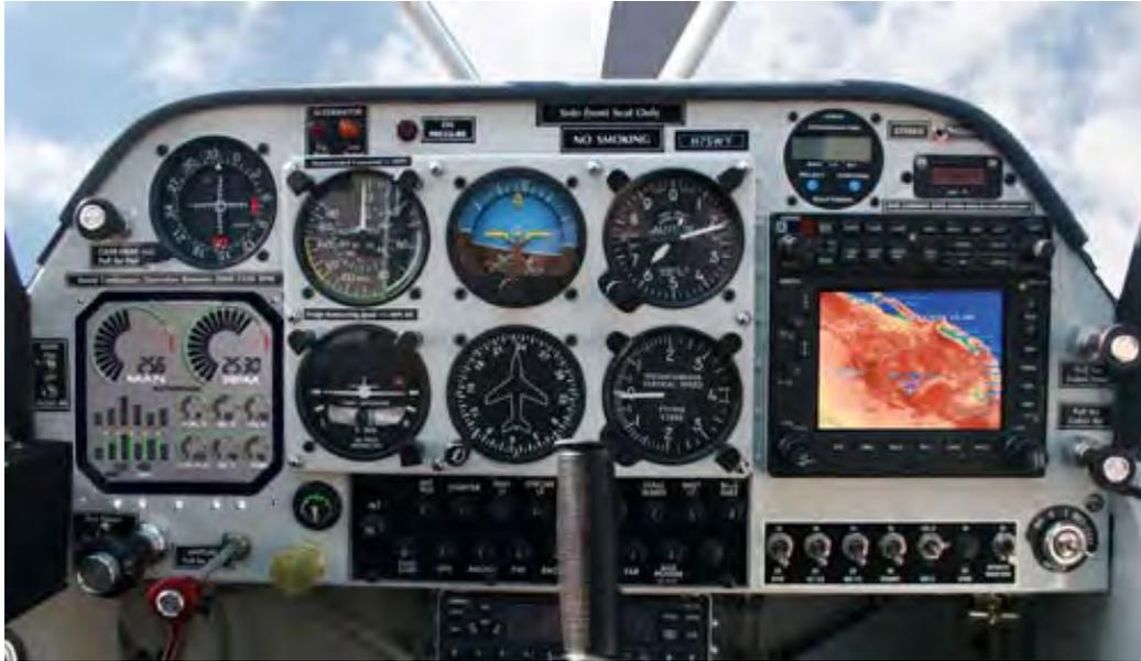
**Figure 18.** A photograph of the exemplar Aviat Husky A-1B instrument panel. (Radio Package 2 panel shown.)<sup>84</sup>
