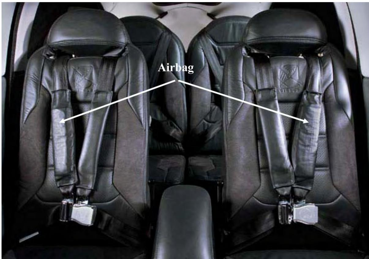
**Figure 17.** A photograph of exemplar Cirrus airplane seats with airbags mounted in the outboard shoulder harnesses.
