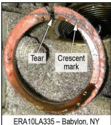
Torn gaskets from three airplanes that lost engine power following oil leaks.
