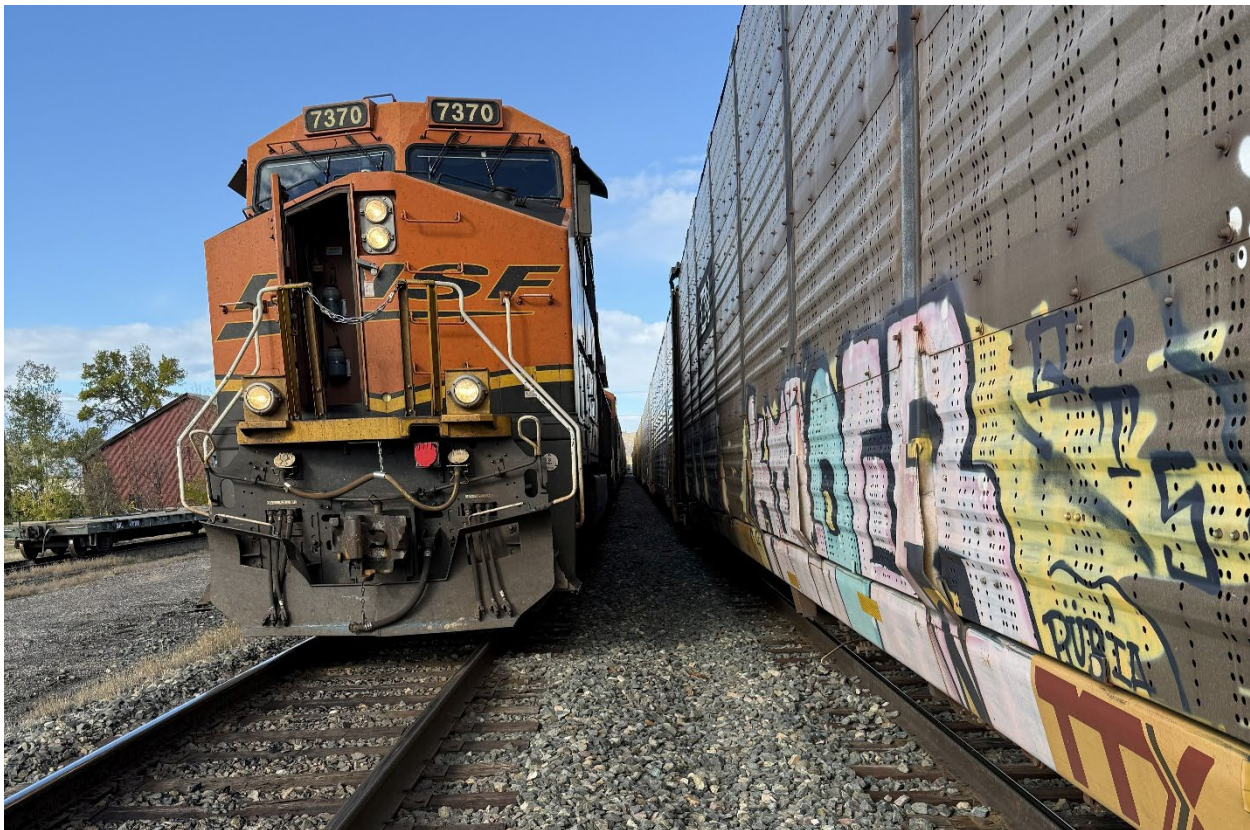
Figure 2. A photograph of the lead locomotive of the striking train staged at the accident location to show the clearance between the siding and the main track.
