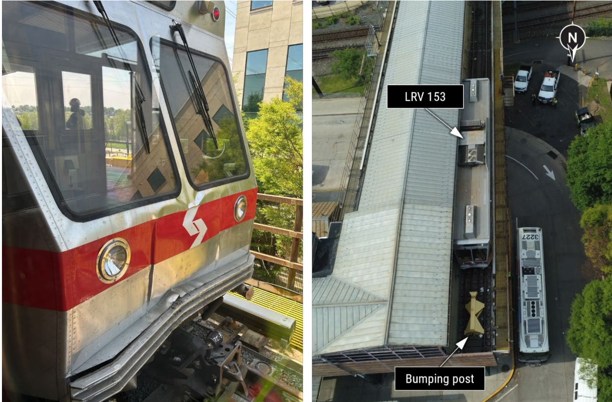
Figure 1. Damaged end of LRV 153 (left) and aerial view of accident scene (right).
