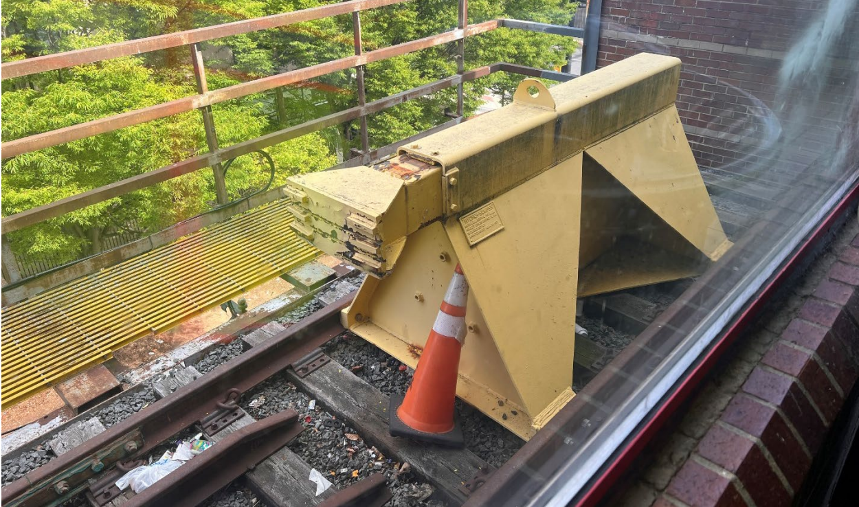
Figure 4. Norristown Station bumping post after collision with the piston driven into the housing.
