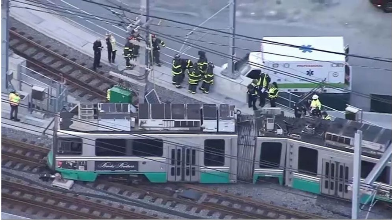
Figure 1. Derailed lead railcar of train 3874-3718.
