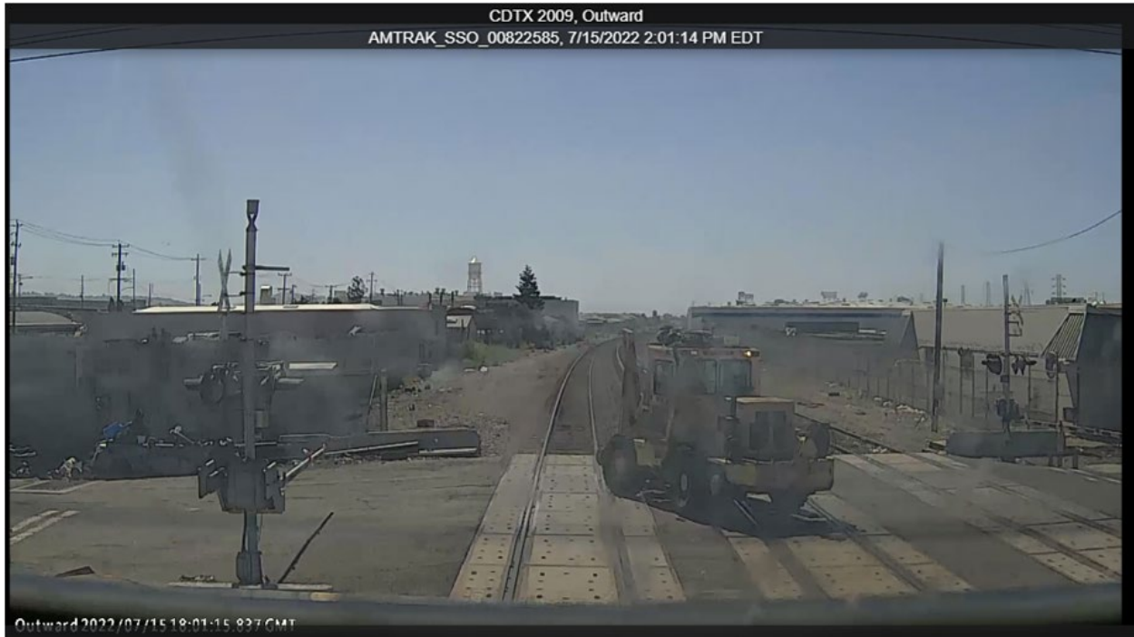
Figure 2. Locomotive image recorder frame showing the RMM shortly before the collision.
