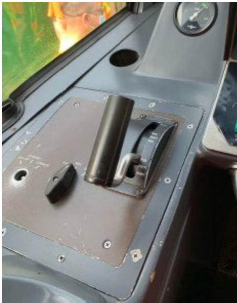
Figure 4. Master controller with deadman's switch disengaged.
