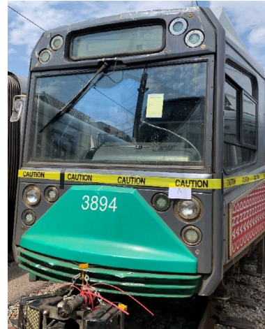
Figure 3. Damage to the front of railcar 3894 (lead railcar of striking trolley).
