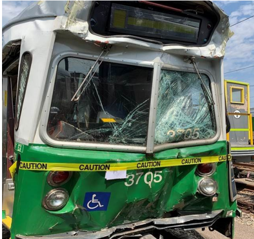
Figure 2. Damage to the rear of railcar 3705 (rear railcar of struck trolley).
