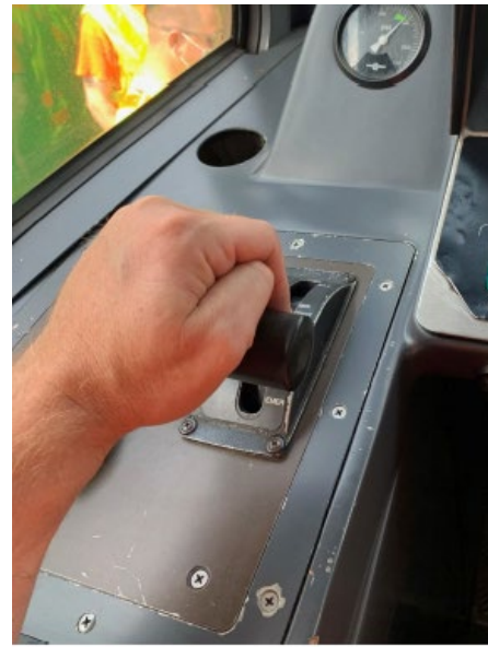
Figure 5. Master controller with deadman's switch engaged.
