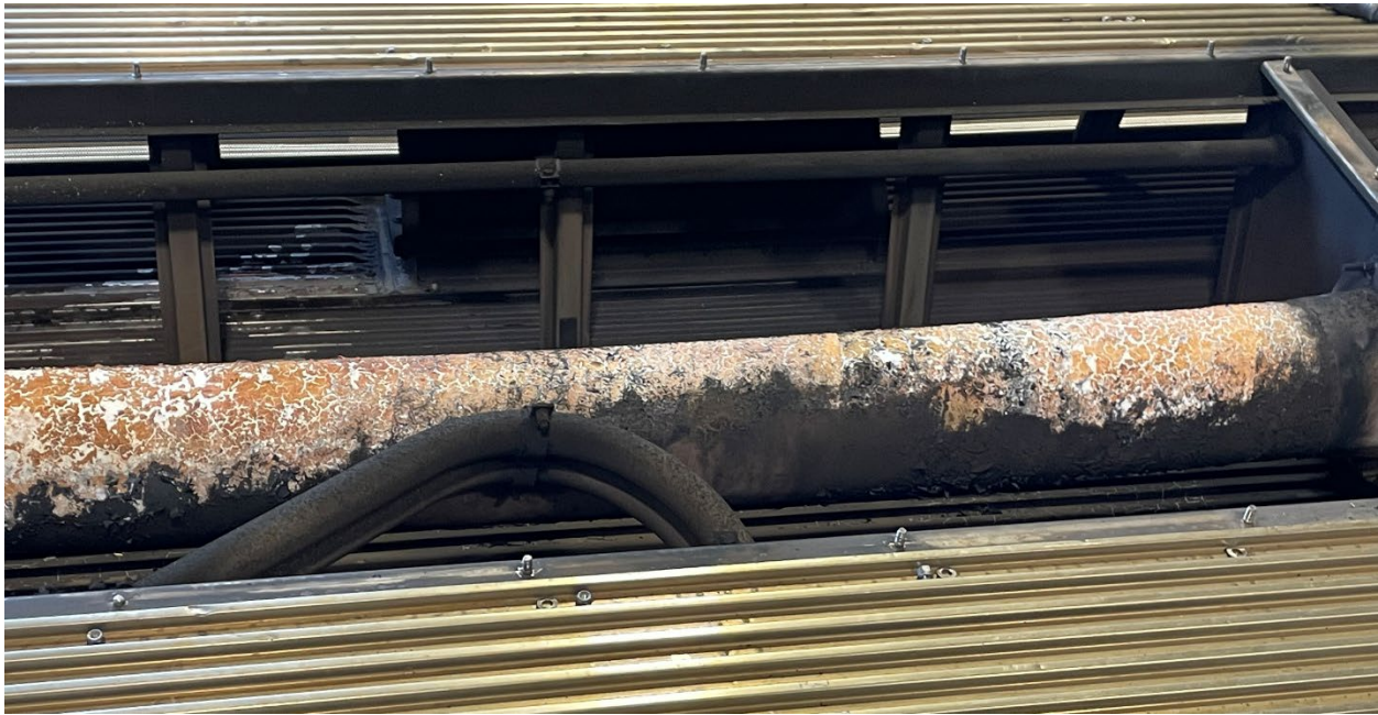
Figure 2. Fire-damaged ventilation duct on railcar following Levittown fire.
