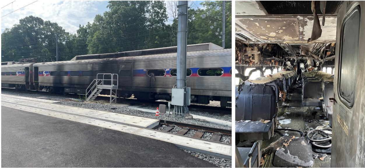
Figure 3. External (left) and internal (right) damage to railcar following Paoli fire.
