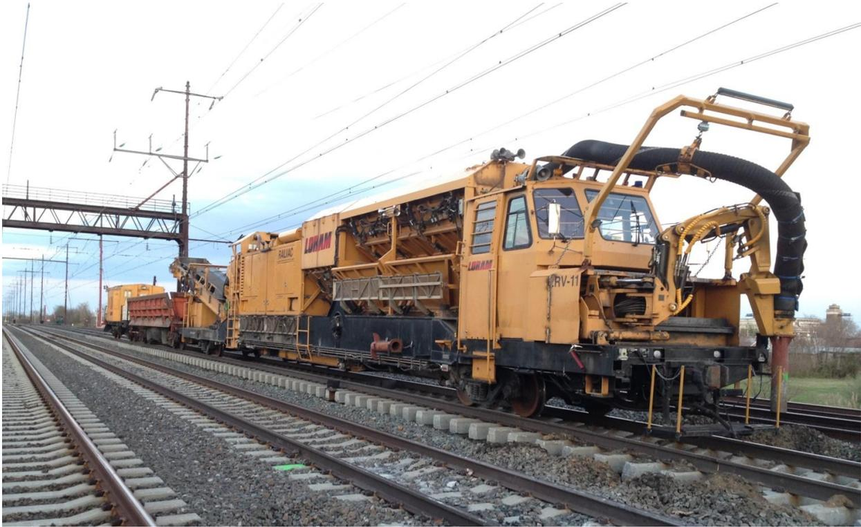
**Figure 2.** RailVac vacuum excavation machine on track 2 at the accident site.
