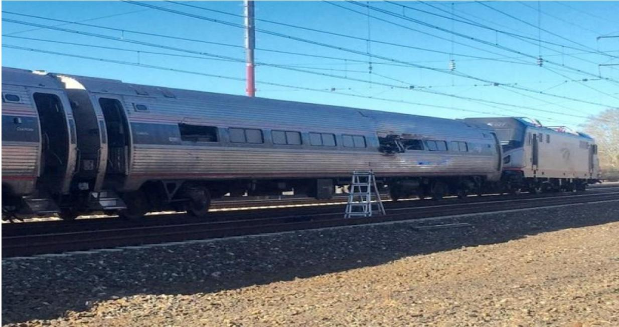
**Figure 9.** Damage to lead passenger car.
