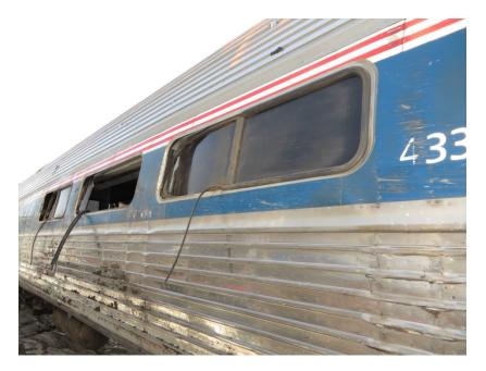
Figure 9. Close-up of damaged windows on right side of car 4.
