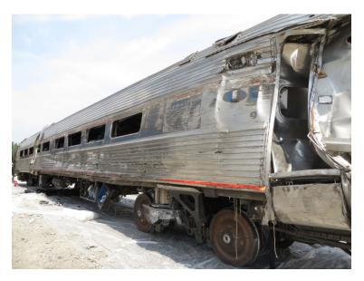
Figure 8. Photograph showing damaged right side of car 3.
