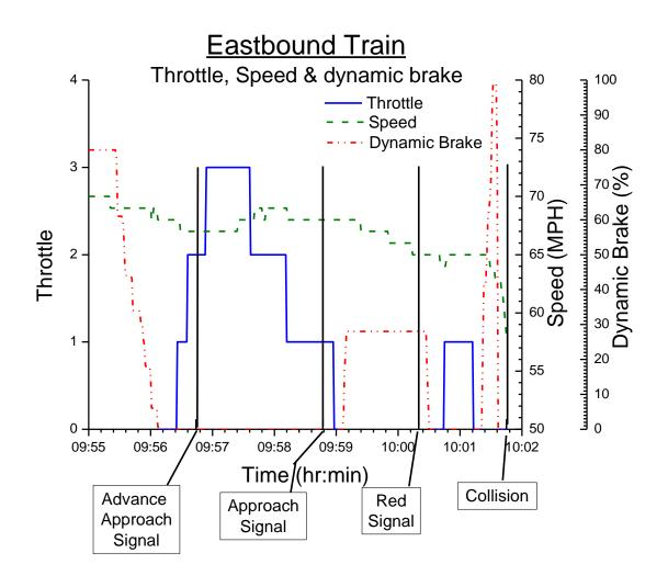
Figure 6. Eastbound train timeline using event recorder data from trailing locomotive.
