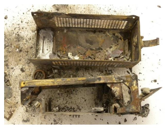
Figure 7. Interior of video recorder hard drive enclosure from lead locomotive of westbound train.
