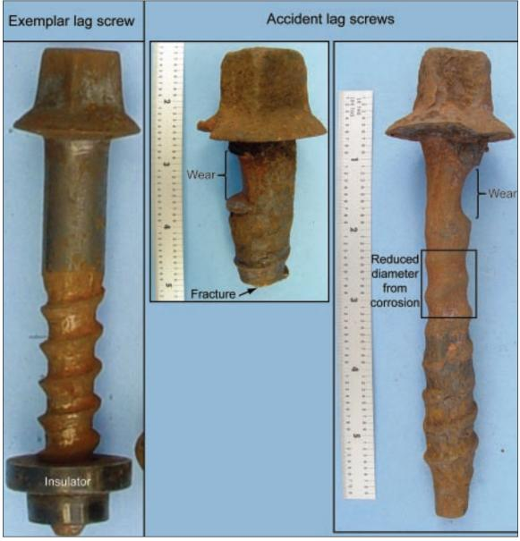
Figure 5. Damaged lag screws from accident location compared to new exemplar lag screw.
