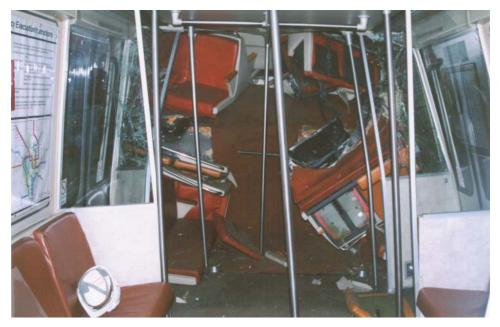
Figure 4. Collision end of car 1077 showing debris field.
