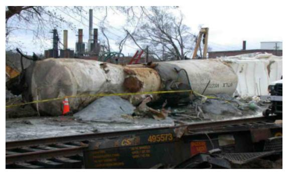
**Figure 8.** Ruptured chlorine tank car during unloading. The tank has been rotated so that the patched puncture is at the top. Hoses attached to the patch are drawing off chlorine vapors that are then bubbled through a sodium hydroxide solution to reduce their hazard.
