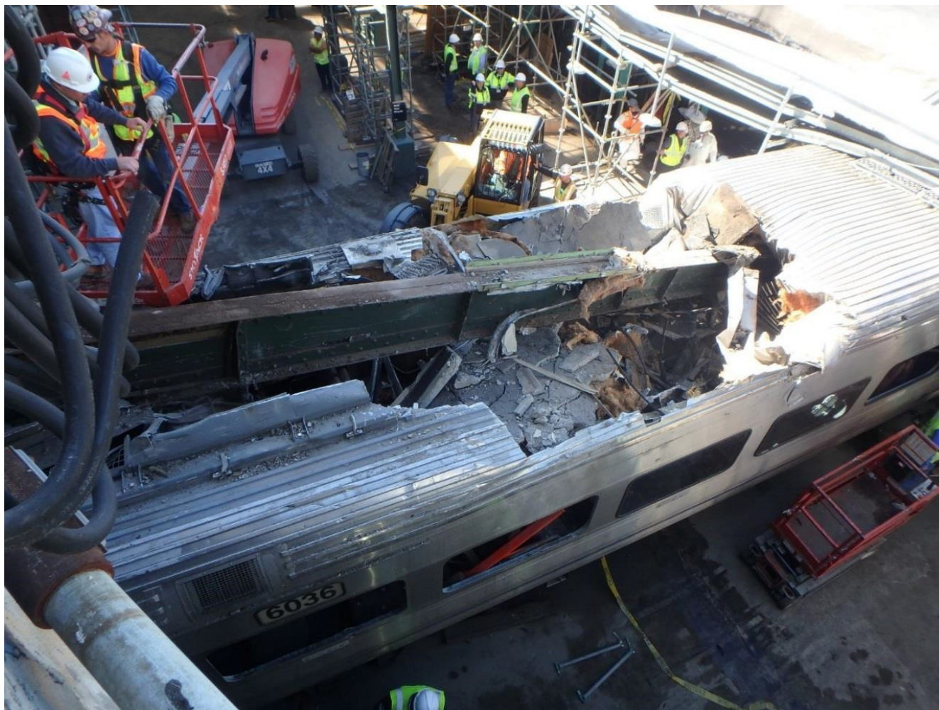
Figure. Damaged controlling cab car.
