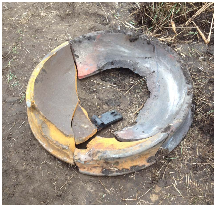
Figure 3. Broken accident wheel at accident site placed as if it were unbroken.
