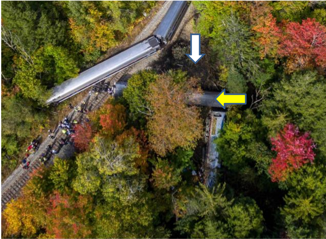
Figure 1. View of derailment (white arrow points to the coach car; yellow arrow points to the locomotive.)
