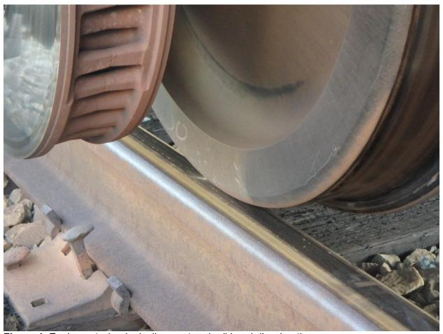
Figure 1. Equipment wheel misalignment and rail head discoloration.
