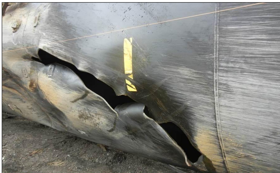
Figure 5. Tear in shell of tank car CBTX 741712.
