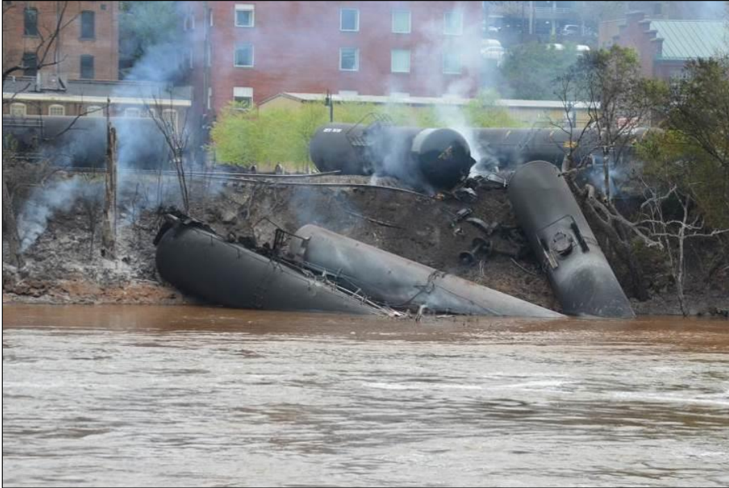
Figure 3. Smoldering, derailed tanks cars on the bank of the James River.
