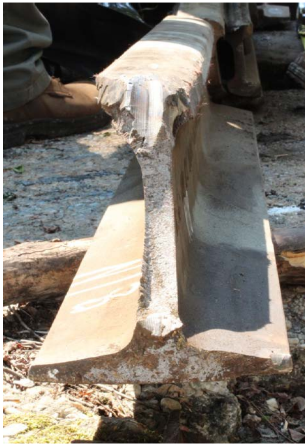
Figure 4. Cross-sectional view of a severe wheel flange strike mark on the head of a broken rail.
