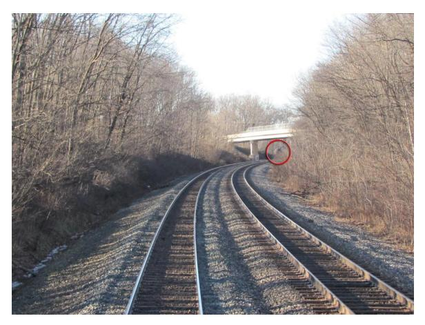
Figure 6. Rear of exemplar standing train (circled) is first visible at about 1,304 feet away.
