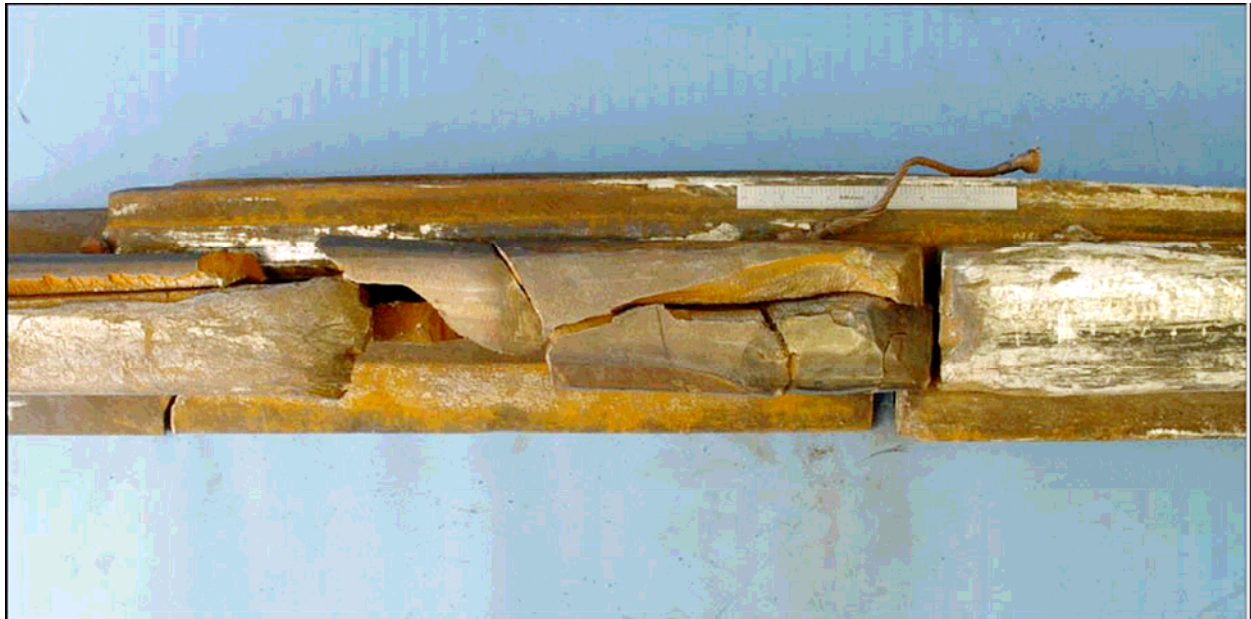
Figure 4. Reconfiguration of plug rail pieces from accident site.
