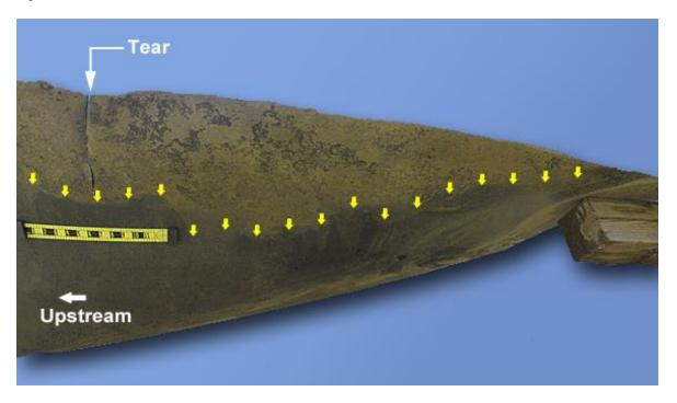
**Figure 9.** External corrosion along longitudinal fracture, with boundary of visible corrosion indicated with arrows.
