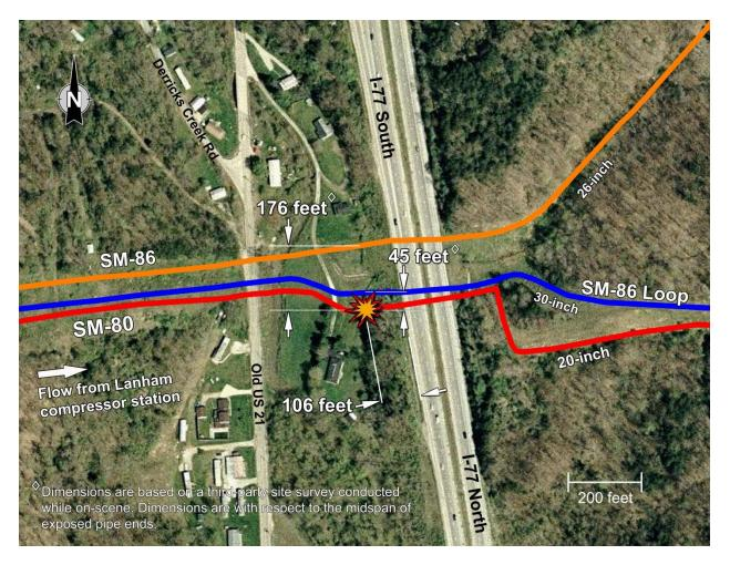
Figure 2. Aerial view of the routes of the three SM-80 system pipelines and the rupture location.
