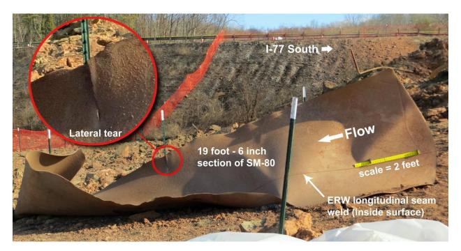
Figure 7. Ejected ruptured pipe.
